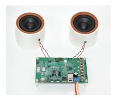
While conventional linear speaker protection algorithms cripple where it matters the most – at high amplitudes - this is where NAU83G60 with KCS truly shines. Its unique feature-set allows operating speakers safely at their physical limits. This enables increased loudness and deeper bass with higher sound quality for consistent best-in-class performance.
